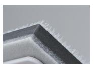
Polyethylene is used for clean use because it does not absorb water
